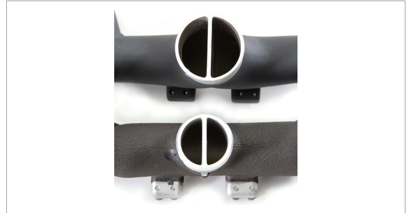
FIGURE 6: Comparison of the stock (bottom) and Mishimoto (top) BOV pipe.
