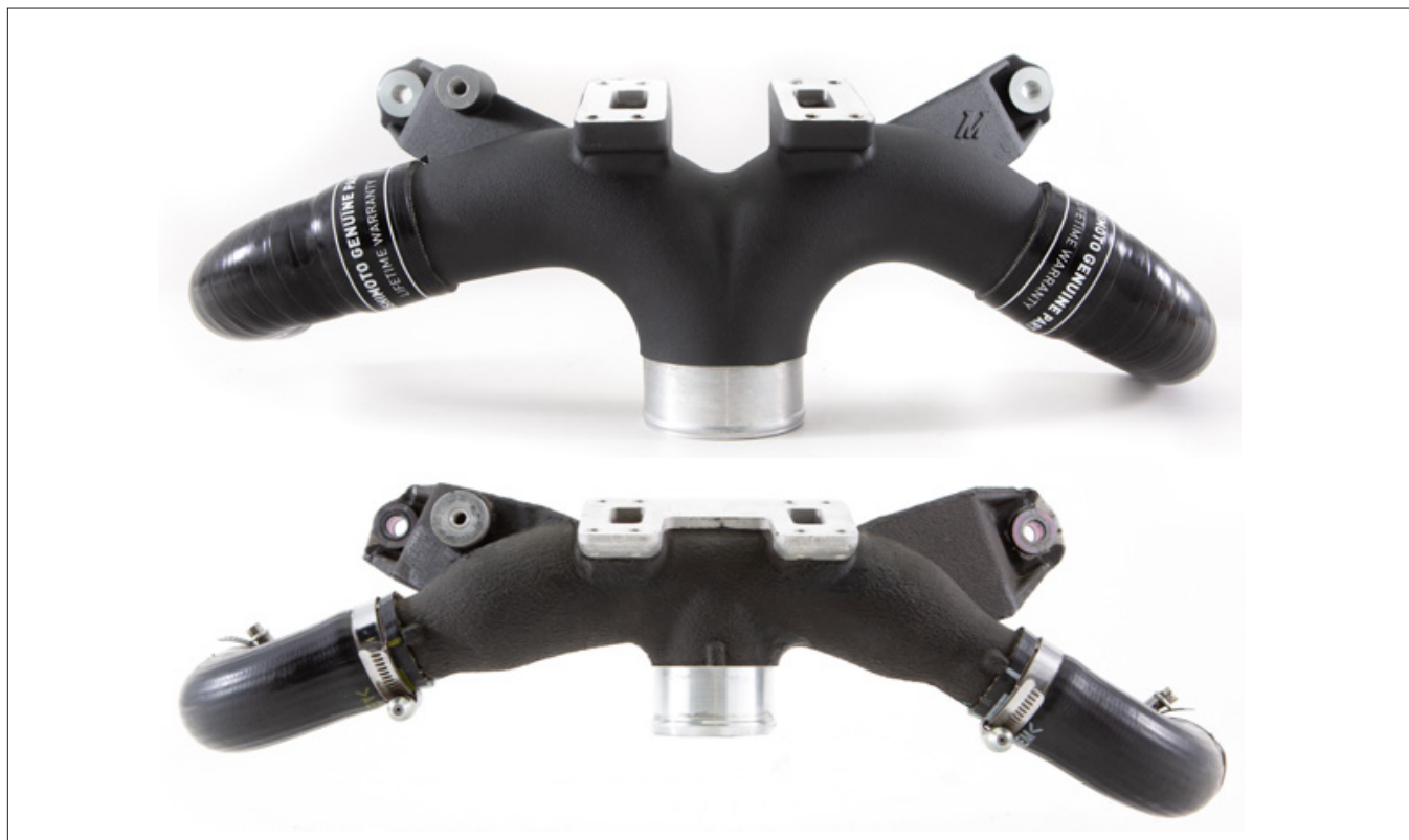
FIGURE 5: Comparison of the stock (bottom) and Mishimoto (top) BOV pipe.
