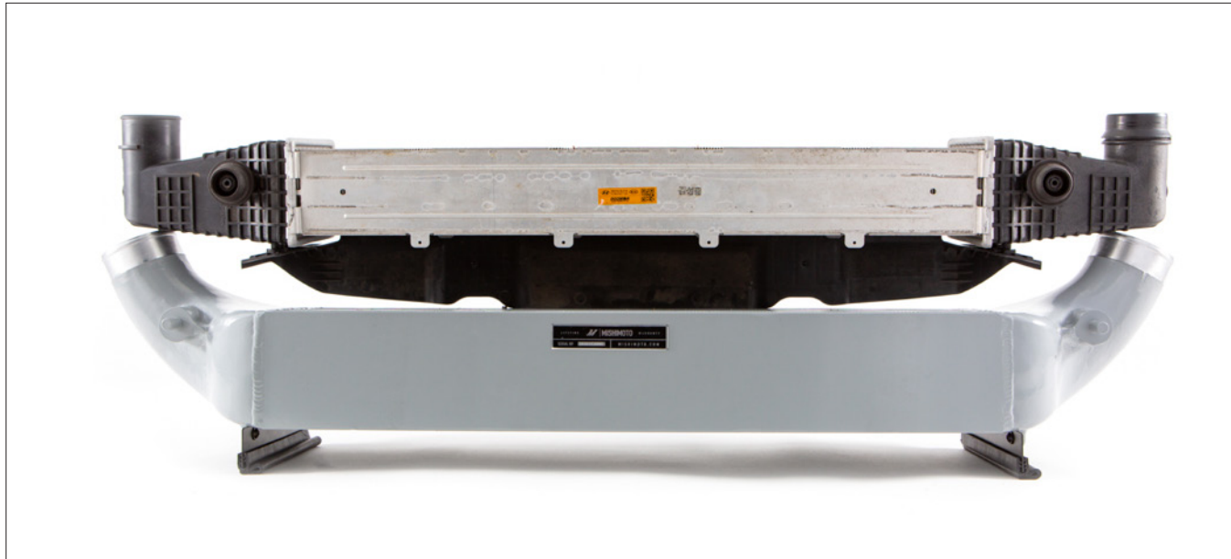
FIGURE 4: Top view comparison of the stock intercooler to the Mishimoto intercooler.
