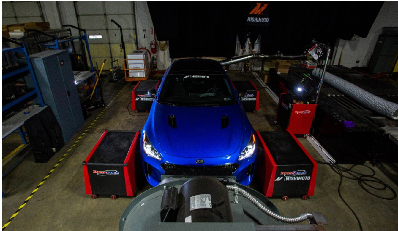
FIGURE 12: A Dynapack dynamometer was used for vehicle testing.
